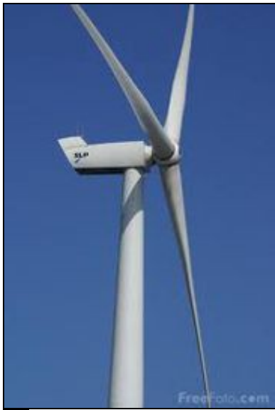
Fig 4(a) Horizontal axis wind turbine
