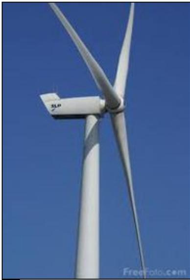
Fig 4(a) **Horizontal axis wind turbine**
