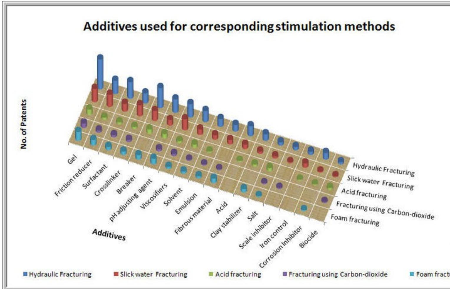
Hydraulic and slickwater fracturing employs viscosifiers for thickening the fracturing fluid which helps in proppant placement but the amount used in slickwater is less as compared to hydraulic as seen in the graph. The highest amount of breakers are used in hydraulic and slickwater fracturing as it degrades the polymers present in the well after fracturing. Friction reducers are mainly employed in slickwater fracturing.
