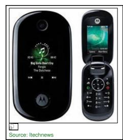
**6. Motorola** - The **MOTO U9** is a Quad-band phone with a 2-inch QVGA LCD display, a 1.45-inch secondary OLED display, integrated music player, Bluetooth, 25MB internal memory and a microSD card slot.
