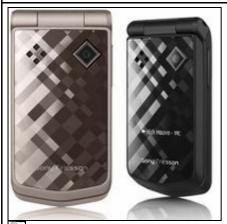
**4. Sony - Sony Ericsson Z555** features a 1.9-inch LCD display, an OLED 128×36 external display, a 1.3 Megapixel camera with 4x digital zoom
