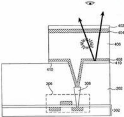
Organic layer emit radiation in all directions, reflecting layer disposed under the anode and reflects the radiation toward the transparent second electrode (Cathode).
