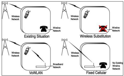
Dual-mode FMC: This form of fixed mobile convergence relies upon dual-mode phones (i.e., mobile cellular and Wi-Fi) and phone-based clients to enable users to seamlessly roam between a wireless LAN (WLAN) and a cellular network. Examples include Agito's RoamAnywhere, and DiVitas' Mobile Unified Communication [Search Mobile Computing]
