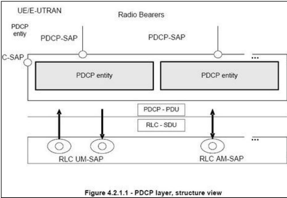
Figure 4.2.1.1 - PDCP layer, structure view
