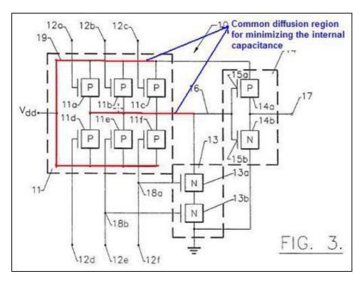
• Internal capacitance of the logic gate also is a major roadblock in increasing its speed. The internal capacitance of the gate also typically limits the number of logic inputs which can be handled by a single gate
