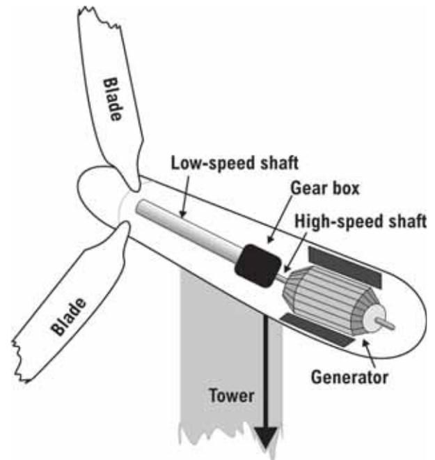
There are many different types of wind turbines with different blade shapes. Wind turbines can be designed to optimize output for specific ranges of wind speed. While one turbine might operate efficiently in winds as low as 2.5 m/s (5.6 mph), another may need winds up to 20 m/s (44.8 mph).
